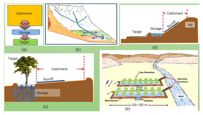
**Fig. 1.** (a) The operation steps of rainwater harvesting; (b) Schematic diagram of macro catchment system; (c) Micro catchment system; (d) Schematic diagram of a macro catchment system with a pond for intermediate storage of runoff; (e) Floodwater diversion under climate change (source: Prinz, 2013)
